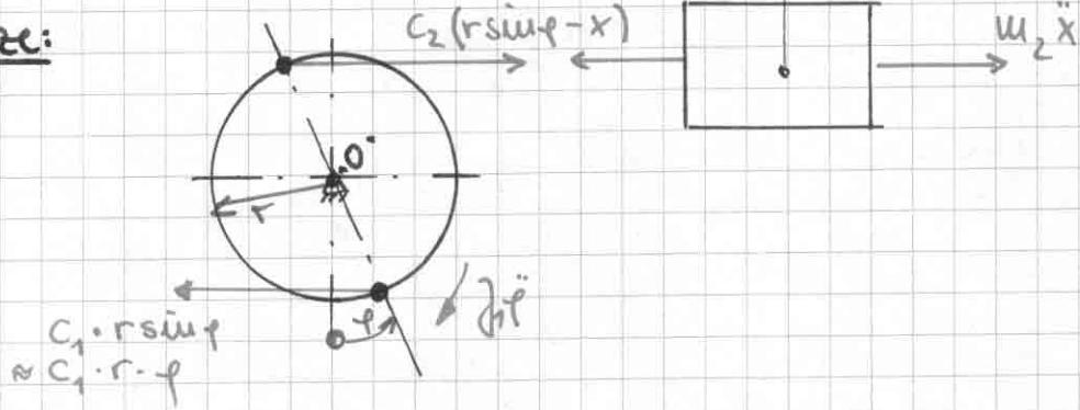
$$\text{DGL: } J_1 \ddot{\varphi} + c_1 r^2 \dot{\varphi} + c_2 (r \sin \varphi - x) \cdot r = 0$$
